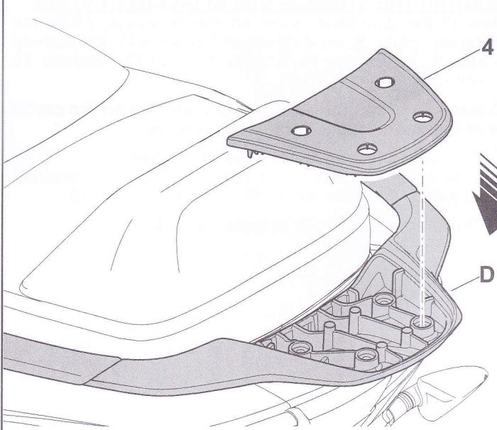
**GB** Place the perforated cover 4 (supplied with the kit) on the socket of the handle D.
