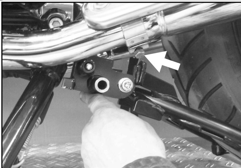
Align the adapter and screw on loosely with the original screw and washer and nut.
