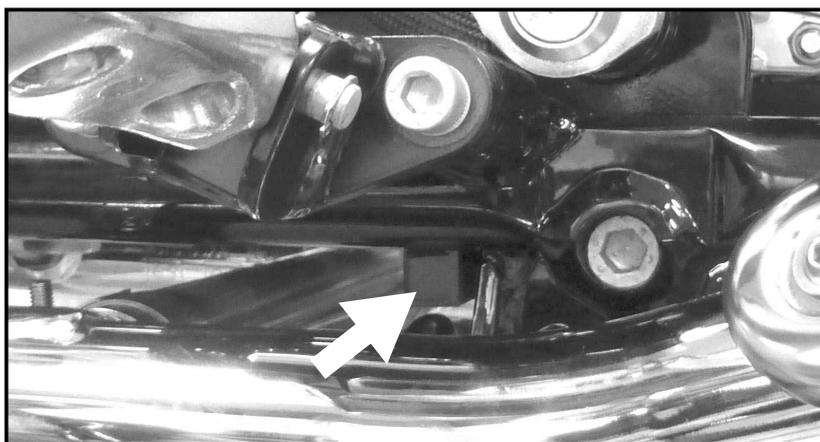
Position the holding adapter so that the previously mounted hexagon screw can be screwed into the open hole on the frame (use small 1/4" ratchet with extension and joint). Slightly tighten the screw.
