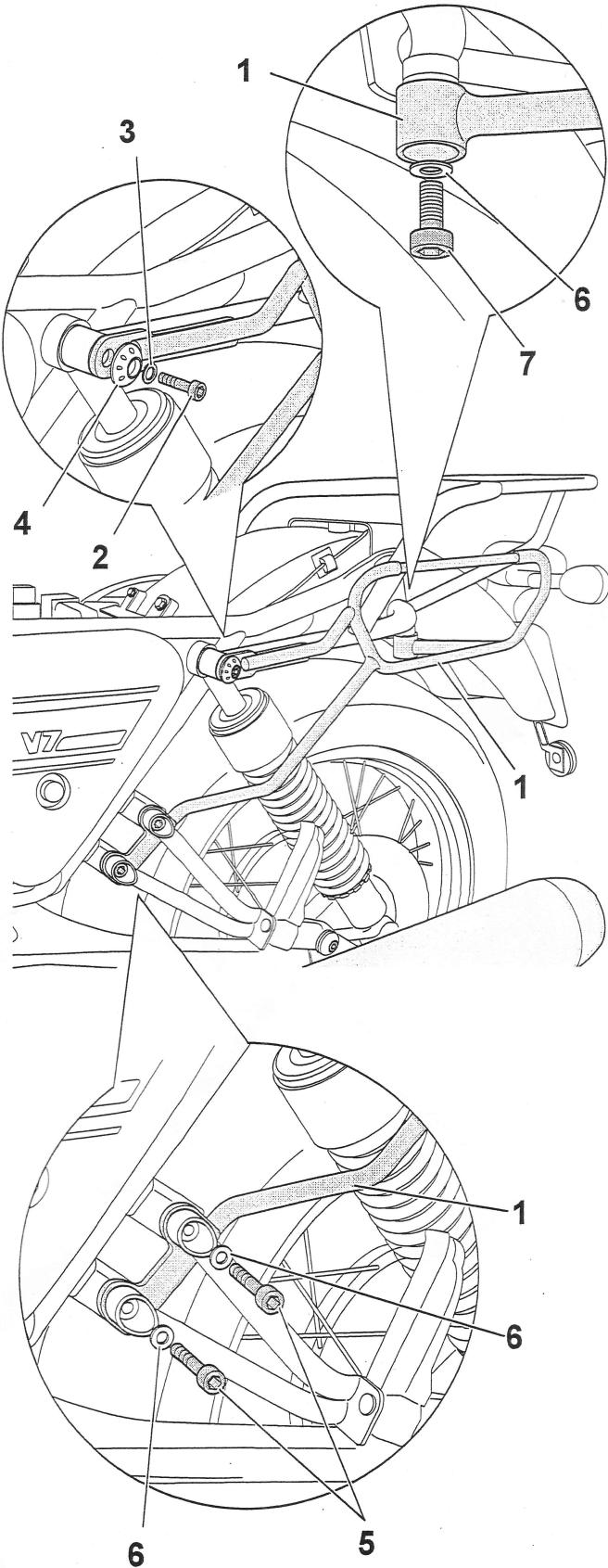
**GB** Position the left-hand luggage rack 1 on the bike, tighten the screw 2 (M6x50) with the safety washer 3 and the aluminium bush 4.
