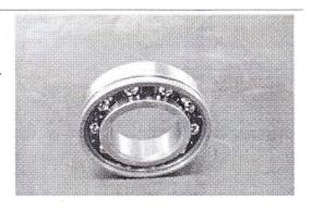
Using the suitable tools, fit the bearing in the crankcase until tool stops
