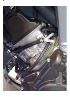
Step Four: Locate the small diameter vent line exiting the LH side of the crankcase (approximately 4 inches to the left of the gear pedal shaft)
