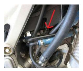
Step Six: Cut the small diameter vent line in approximately the middle and re-route as necessary to install the "Y" union as seen in the photo below
