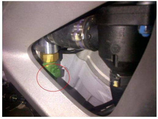
15. Remove the original manifold from the bike; using tools "F" and "G" unscrew the temperature sensor:
