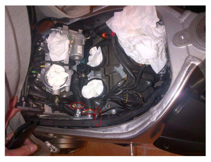
13. Remove the coolant: open the radiator cap and the expansion vessel cap.
