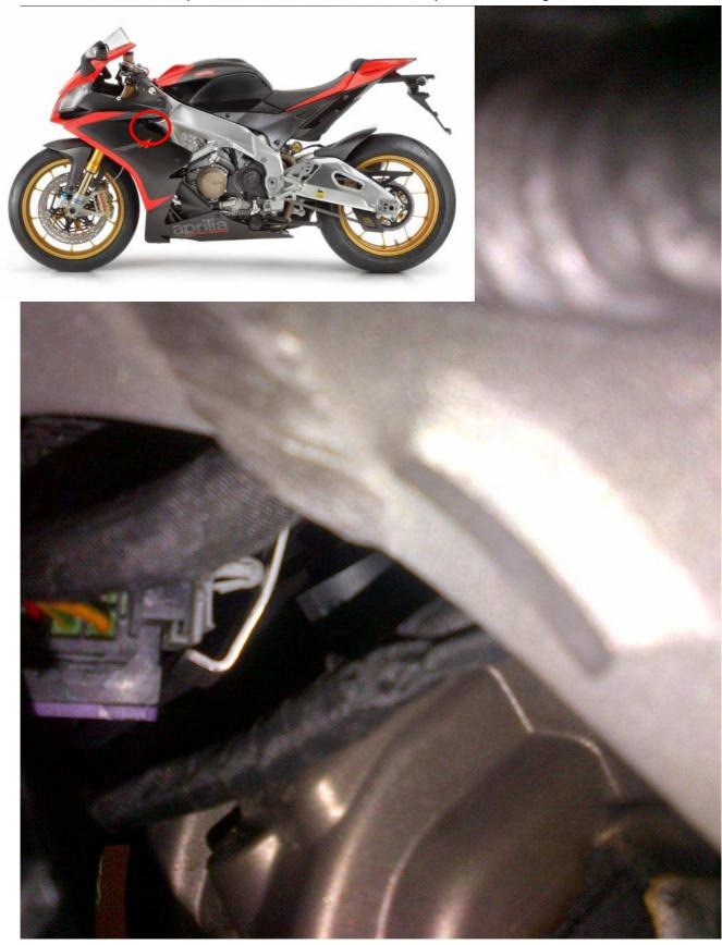
6. On the left and right side of the airbox, you can find intake sensors for front and rear cylinders. Using tool "C" unscrew them from the airbox.
