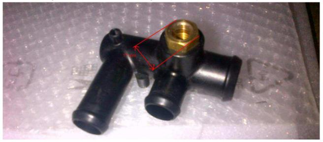
16.Install the sensor on the cnc manifold:
