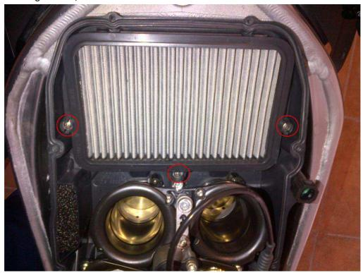
3. Using tool "A", unscrew the 4 screws with cylindrical head that fixes the variable geometry trumpets on the airbox (BE CAREFULL: remove exactly the 4 screws circled in red; don't touch the others!):
