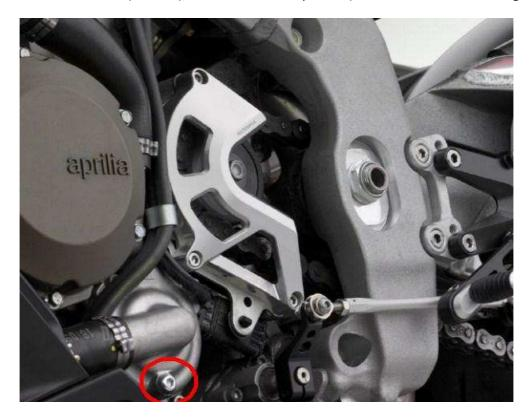
14.At this point you can remove the original coolant manifold: open the three "Click" clamps using tool "D" and disconnect the temperature sensor:
