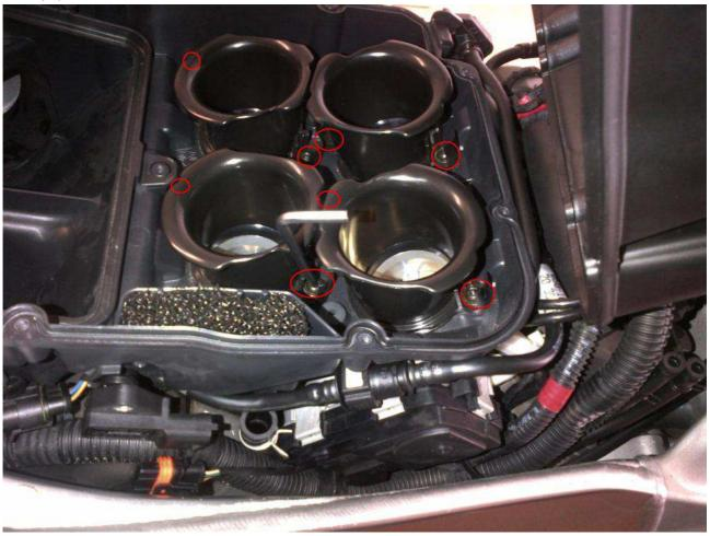
8. Lifted the rear side of airbox, is possible to remove it (be careful to don't pull connectors or wires!)
