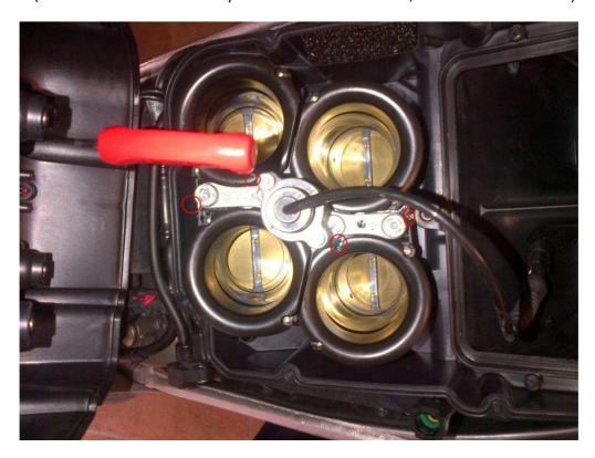
Remove the variable geometry connector from the airbox cover.
