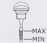
Since a certain quantity of oil still remains in the circuit, oil must be filled from oil dipstick/cover.
