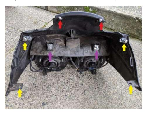
The red arrows point to two Phillips screws along the top of the dashboard. Remove those. The upper yellow arrows are easily visible and accessible. Remove those.
