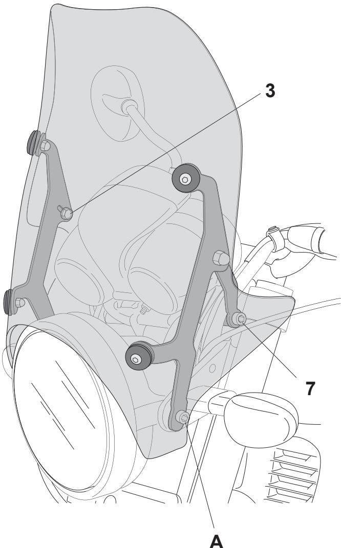
**G** Partially screw in bolts **7** TCEI M8x40 to secure supports **1** and **2** to the bracket ignition switch block.
