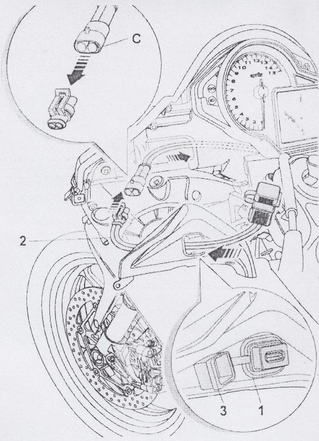
From the front of the grill, insert the cable 2 of the USB 3 port into the hole of the rubber 1 and insert the port taking care that the door opens to the left (the longer side of the grill).
