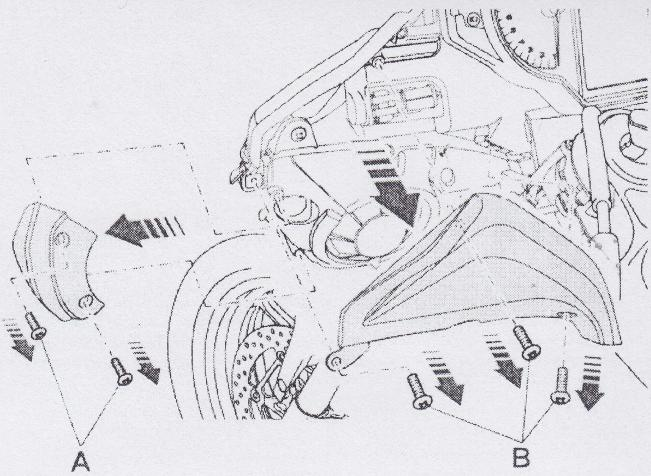
Unscrew and remove the fixing screws A and remove the side grill.
