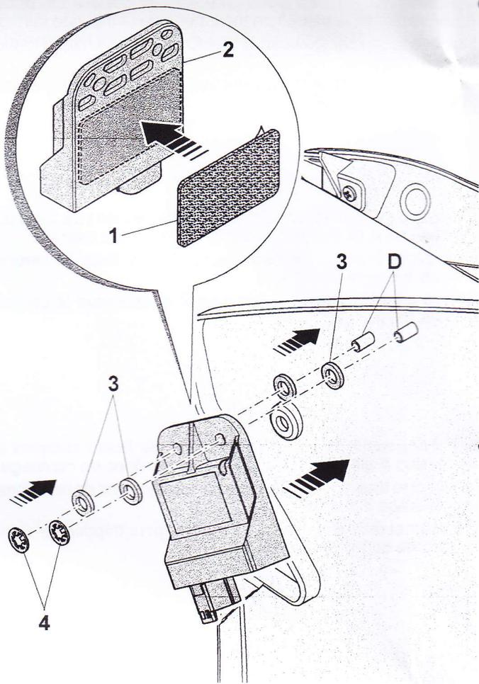
**GB** Apply the expansion adhesive rubber 1 on the lower part of V4-MP control unit 2.
