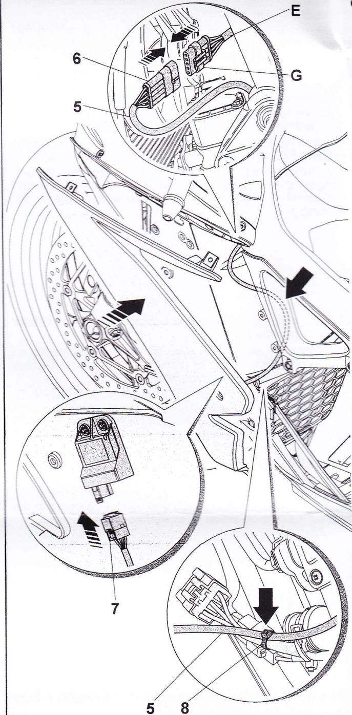
**GB** Connect the connector 6 of the control unit wiring harness 5 to the connector G of the wiring harness E on the vehicle.
