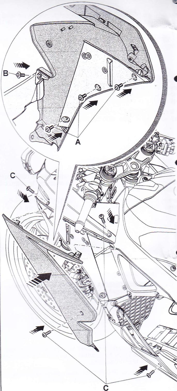
**E** Place the left side fairing again on the vehicle, first engage it to the top fairing and then fix it with the relative fixing screws C.
