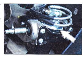
9. Lock the screw securing the top of the side sleeve to the parallelogram at a torque of 45 ÷ 50 Nm.
