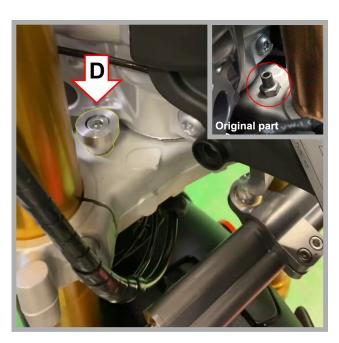
**A)** Mount the triangular support on the frame, above the lower steering plate. **B)** Mount the steering damper on the support. **C)** Extract the steering damper arm, than lock its spheric bearing to the lower steering plate end, inserting the bushing first and then screwing the long screw into it. **D)** Remove the original travel stop bolts placed between chassis and swingarm, and replace them with the bushings, using the screws.
