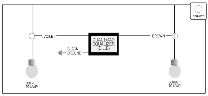
The Dual-Load Equalizer is designed to fix the problem when you have changed your stock directionals to L.E.D. turn signals and they flash quickly or not at all. It will equal the load that your system expects from the original incandescent bulbs by evening the load being sent and ultimately allow your signals to work properly.
