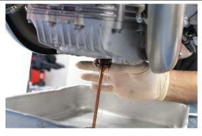
Once the oil has drained out, screw in and tighten the drain plug with its washer to the prescribed torque.
