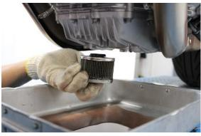
When reassembling, use a new O-ring seal for the engine oil filter cover.
