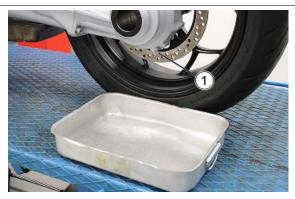
Loosen the drain plug without removing it.
