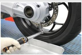
Using a special syringe, fill in with new oil through the filler cap.
