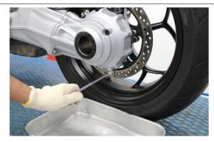
Unscrew and remove the filler plug (2).
