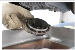
Screw in and tighten the 3 fixing screws for the engine oil filter cover to the prescribed torque.
