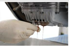
Remove engine oil filter cover with the spring.
