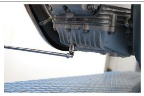
Place a container with adequate collecting capacity at the engine oil filter cover and completely unscrew the 3 fixing screws.
