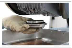
Remove the engine oil filter.
