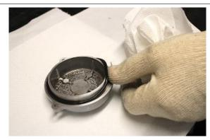
Insert the new engine oil filter.
