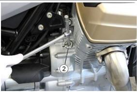
Unscrew the drainage cap.
