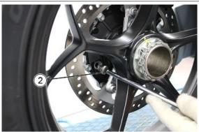
Completely unscrew and remove the drain plug. Drain the oil into the container for at least 5 minutes for oil to drain out completely.
