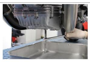
Remove the drain plug and allow the oil to drip into the container for a few minutes.
