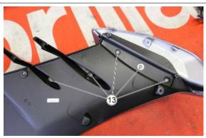
Separate the winglet (14) from the outer part (15) of the side fairing.
