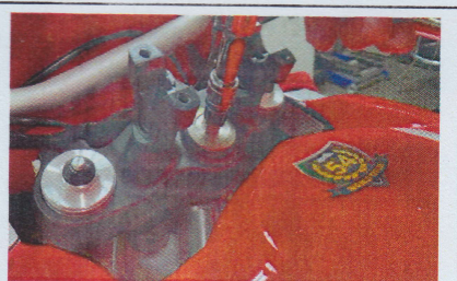
Remove the main triple clamp nut with a 12mm allen socket.
