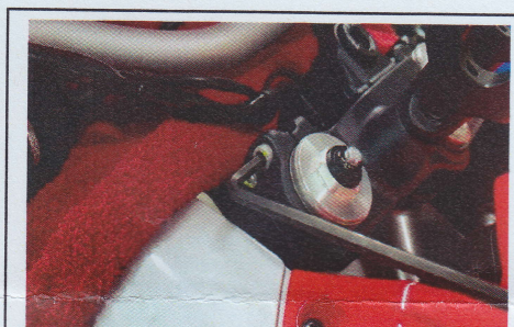
Remove upper triple clamp pinch bolts & put one aside for a reminder they're loose
