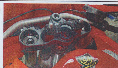
Step #12 Install the Scotts base plate over the studs so the recess on the plate matches the flange on the stud.
