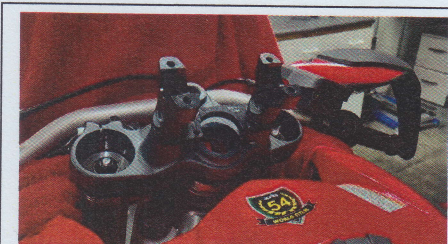
#13) Thread the lower perches onto the studs, hand tight, roughly aligned so you proceed to the next step.
