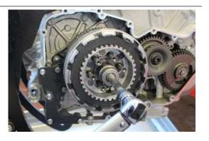
• Insert the disc with friction material and the black tooth into the bell.
