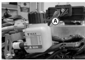
Unscrew and remove the plug (A).
