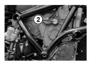
Unscrew and remove the plug (2).
