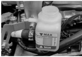
Begin filling the inverter cooling system by pouring the liquid coolant indicated in the fluids table (0.4.3) into the tank.
