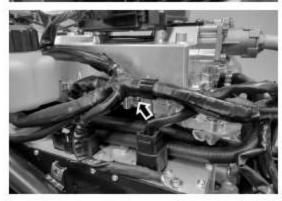
Unscrew the indicated bleed screws on the left and right hand side of the inverter.
