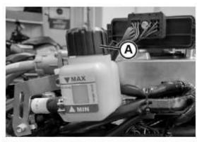
Unscrew and remove the plug (A).
