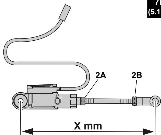
**GB** Remove the lower joint with left-hand thread (**M1**) from the standard gearshift rod (**M**) and assemble it on the gearshift rod (**2**) of the kit. Assemble the quick shift device (**1**) and the gearshift rod (**2**) of the kit, adjusting the distance between the centres to the same measured during the disassembly of the standard rod (**X mm**). Having adjusted the length of the rod, tighten the locknuts (**2A**) and (**2B**).
