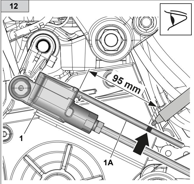
**GB** Using a felt-tip pen, mark a reference at 95 mm on the cable (1A) of the quick shift device (1).
