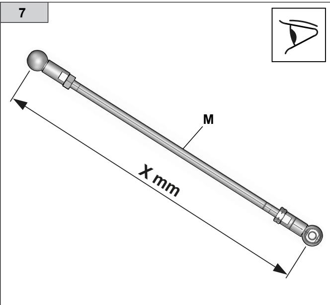
**GB** Measure the distance between centres of the series (**M**) gearshift rod and note the measured value (**X mm**).
