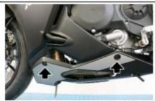
Slowly lower the lower fairings, pulling out the breather pipe at both the front and the rear.
