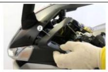
Remove the outer fastener screw of the upper fairing trim piece (3).
