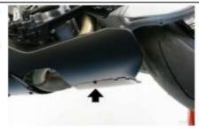
While supporting the weight of the lower fairings, remove the lateral fastener screws on both sides.
