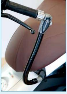
605537M017 Mechanical anti-theft system for connection of the handlebars to the chassis. Consists of a rotating head and internal steel cable. All made from hardened steel.
