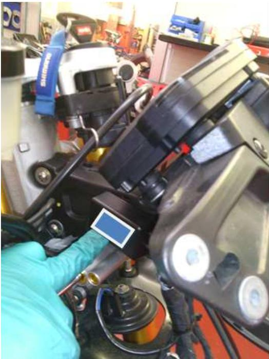
3.7 Fix the Blipper WHITE Main Board on the left side below the dashboard
